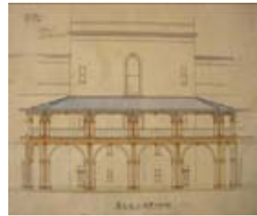
Figure 55: Addition to the back verandah, 1891, which linked the existing rear verandahs following demolition of the refreshment rooms. The drawing shows a timber structure with a cast iron balustrade and is signed by H.A. Still.
