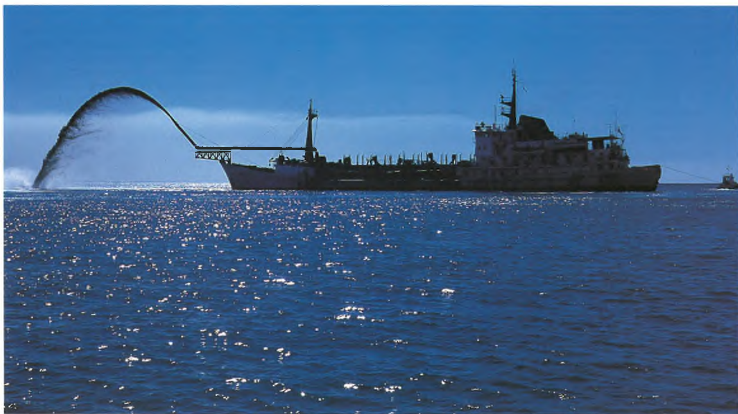
The Port of Brisbane Authority's dredger Sir Thomas Hiley pumps sand as part of a trial beach nourishment program.
