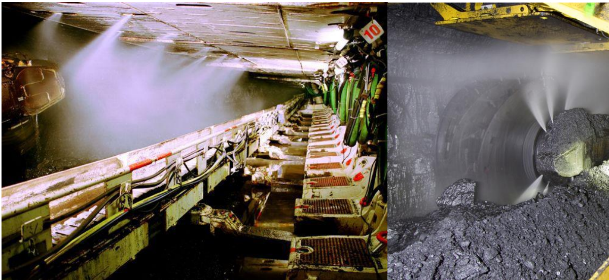
Image 10 Shield canopy sprays and ranging arm sprays
