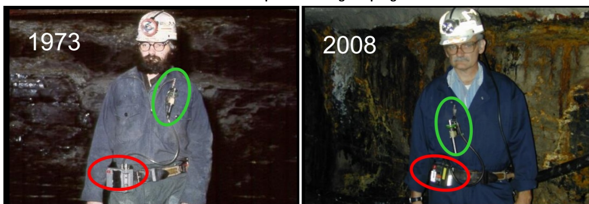
Image 14 Gravimetric dust sampling technology, 1973 and 2008 Same USA miner depicted wearing sampling devices
