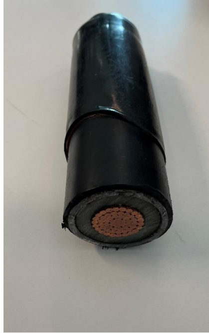
Example of 11,000 volt electricity copper cable
