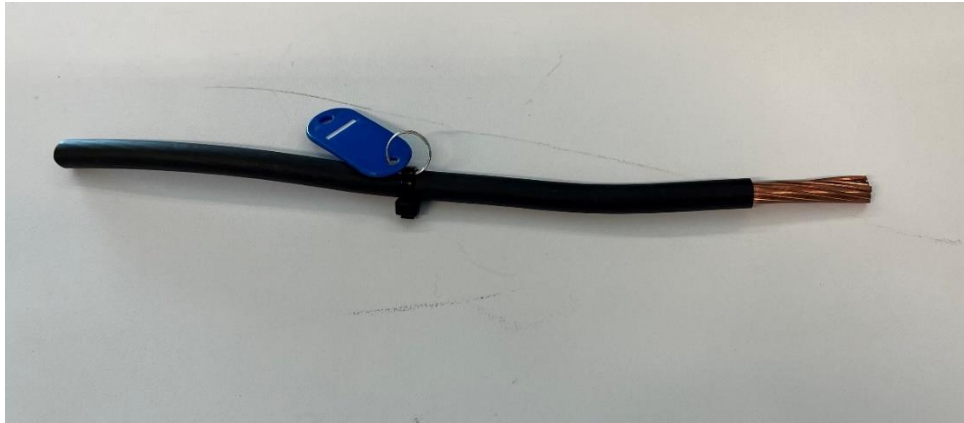
Example of copper neutral earthing wire
