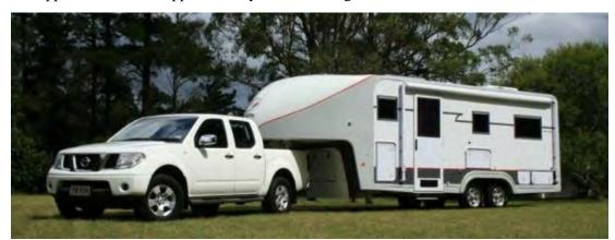
[3] Our single unit motor-home. 8.7metres long GVM exactly 5 tonnes and with 6 road wheels [some similar motor-homes would have just 4]. There are only 2 axles, not 3, even though there are 6 wheels.
