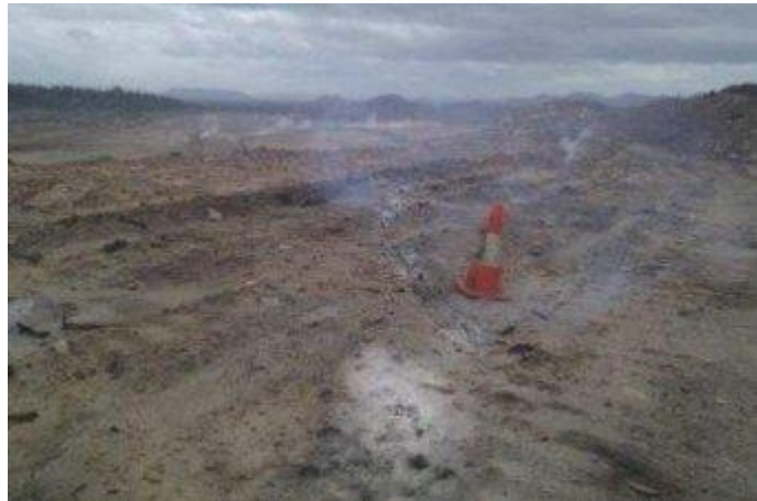
Figure 2. Gas rises from the ground at the Collinsville open cut coal mine (from Wordsworth, 2012).
