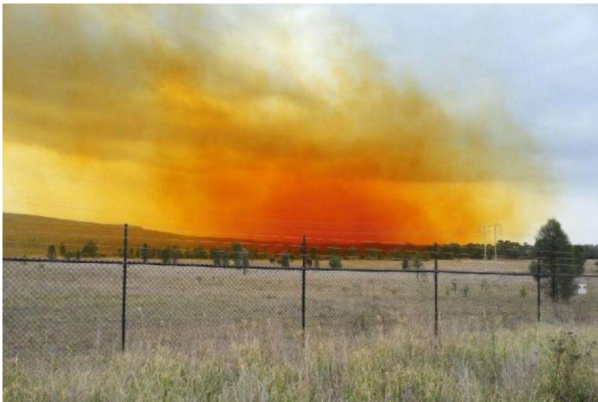
Figure 1. Orange blast fume plume over Muswellbrook after a blast at BHP's Mt Arthur Coal Mine (from Lamacraft, 2014).
