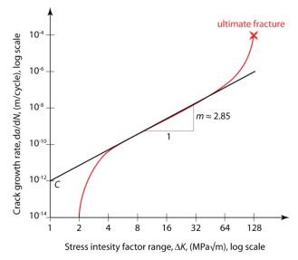
According to the image on the left, as the stress intensity applied upon the material increases, so does the crack growth rate. There is a gradual increase in crack growth from between 4 to 50 MPaVm of stress intensity but after around 50 MPaVm, the crack growth steeped to the ultimate fracture. The danger in taking a risk on lifters, is that no one can accurately predict the crack growth rate of the lifter and neither can anyone predict when it will snap.
