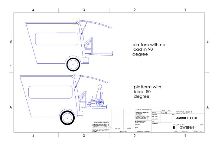
As the above drawing illustrates the lifter will be 90 degrees to the arm but when a load is applied to the lifter it becomes stressed and reduces by 10 degrees. Over time one can see this movement having an impact on the strength of the lifter and signs of steel fatigue become evident.
