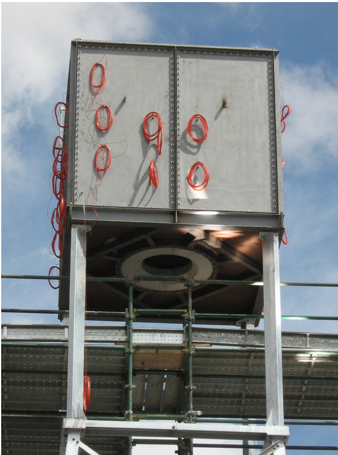
Close up of solar receiver at base of storage/boiler unit
