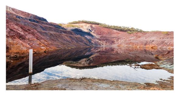
The solution is likely to be relatively simple – backfill the pit with the acid forming waste material and cap the site with a fit for purpose cover. However, a combination of lack of funds and the desire to keep the site open in case a future buyer is found, means the site continues to contaminate the environment.
