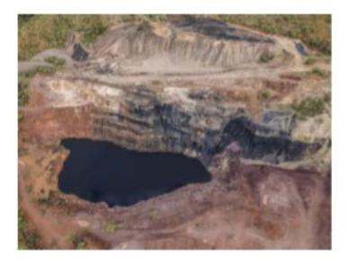
The pit remains open and after significant rain fall events, acidic water escapes into surrounding creeks. With a pH of 2 the water quality in the pit is similar to battery acid. The site has been leaking acidic water laced with heavy metals into the environment since the 1960s and the situation continues with no genuine attempt to rehabilitate the site.
