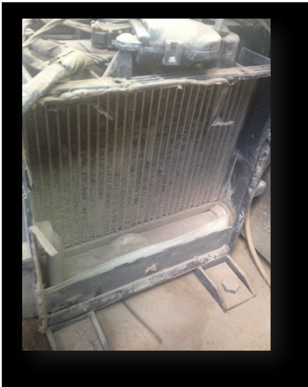
Picture 1. OEM filter HVAC system internal components covered in dust . Accumulated over time eventually causing HVAC maintenance due to poor performance and/or HVAC failure.
