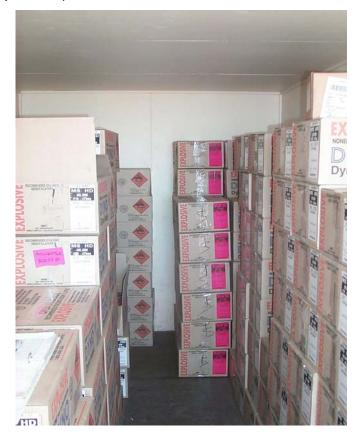
Figure 10: Explosives stacked with their labelling towards the access way for easy identification.
