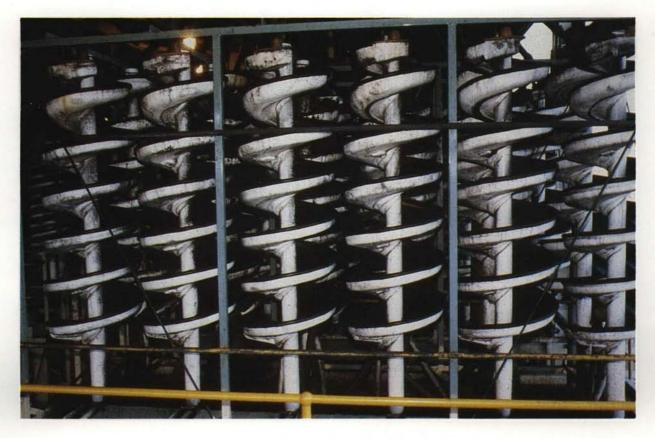
Preparation plant German Creek – spiral concentrators for treatment of fine coal in the 0.5–0.1 mm range.
