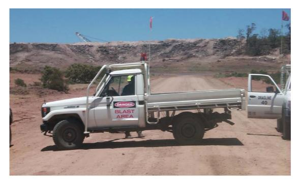
Figure 13: Access guard with signage
