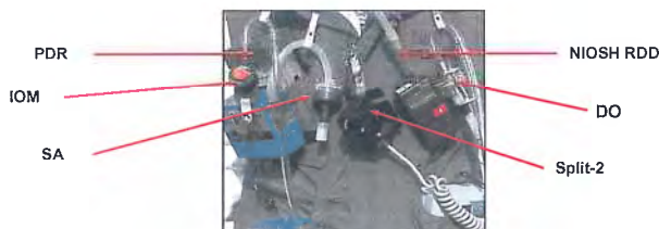
Figure 3: Sampling harness with six personal dust monitors
