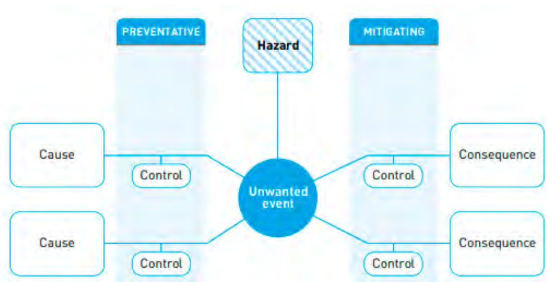
Figure 29: Simple bowtie diagram
